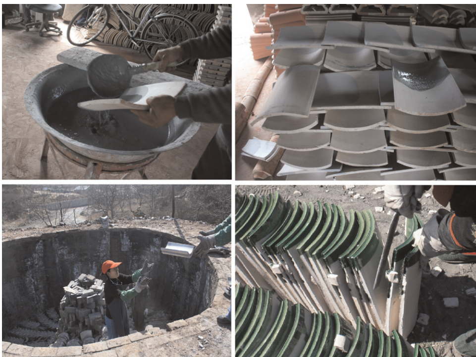
Fig. 9. Production sequence for glazing tiles in Liuli Village, Beijing: (top left) pouring glaze from a ladle; (top right) drying flat tiles; (bottom left) stacking tiles vertically in a kiln; (bottom right) chopping out ceramic separators between tiles (photos by Wong Wai Yee Sharon).
